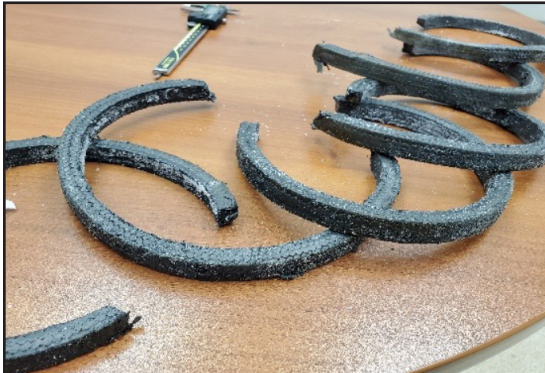
Old rings of failed anti-keystone packing.
